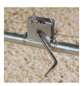
Single handle adjusts cones on 300 feet (92 meters) of feeder line.
